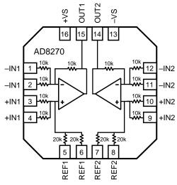
Figure 1. AD8270 Dual Difference Amplifier
